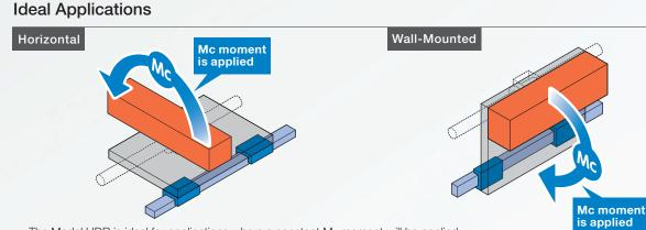
The Model HDR is ideal for applications where a constant  $M_c$  moment will be applied, such as configurations where an object will hang over the side of the table, or where the table is wall-mounted.
