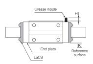
Location for mounting the side grease nipple
