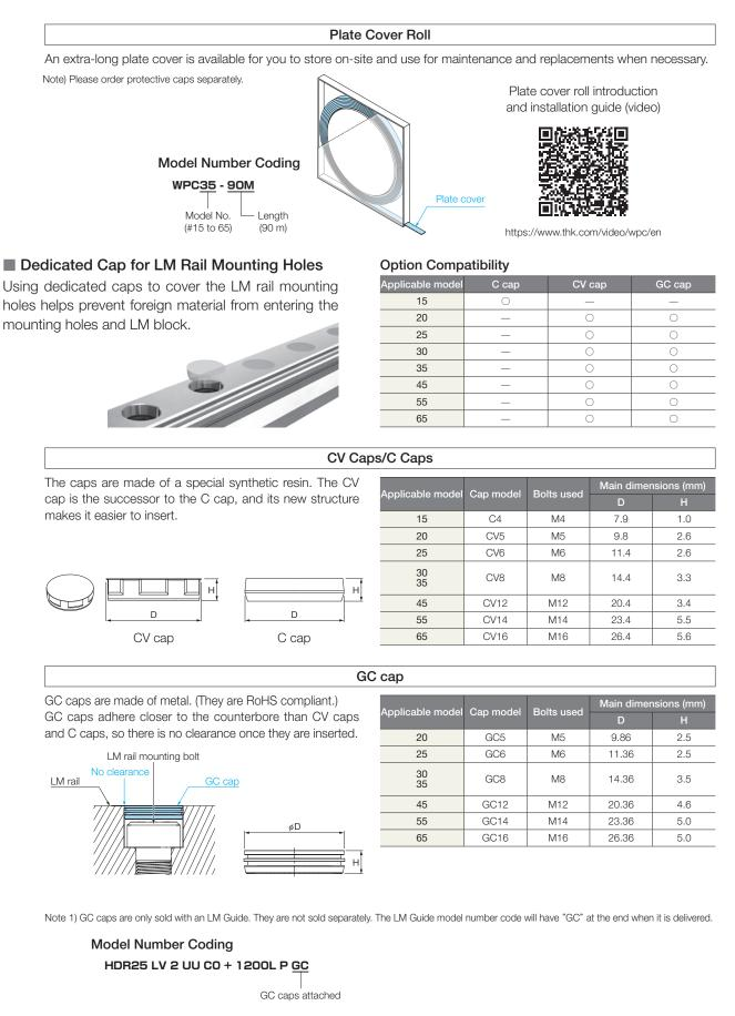
Note 2) GC caps cannot be used with LM rails that have undergone surface treatment.
