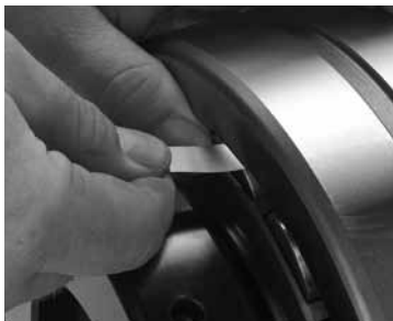
Fig. D-7. Measure RIC before installation.
