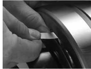
Fig. D-3. Measure RIC before installation.
