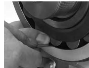
Fig. 4. During mounting, the RIC should be checked at the unloaded roller.
