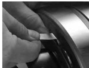
Fig. 3. Measure RIC before installation.
