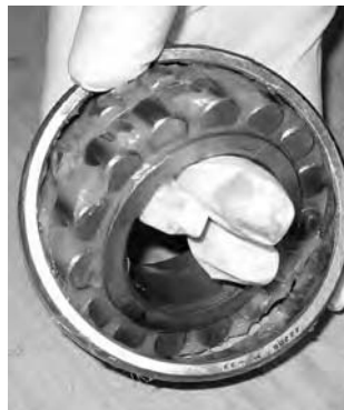
Fig. 10. Grease can easily be packed by hand.
