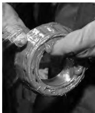
Fig. 147. Grease can easily be packed by hand.
