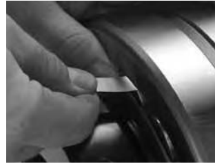
Fig. 91. Measure RIC before installation.
