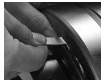
Fig. 95. Measure of RIC before installation.
