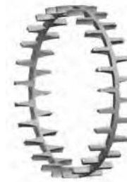
Fig. 45. One-piece, machined-brass, land-riding, finger-type cage.
