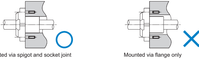
Mounted via spigot and socket joint
