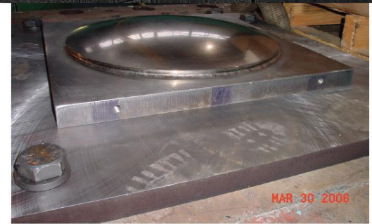
Figure 9-5 Convex and masonry plates.
