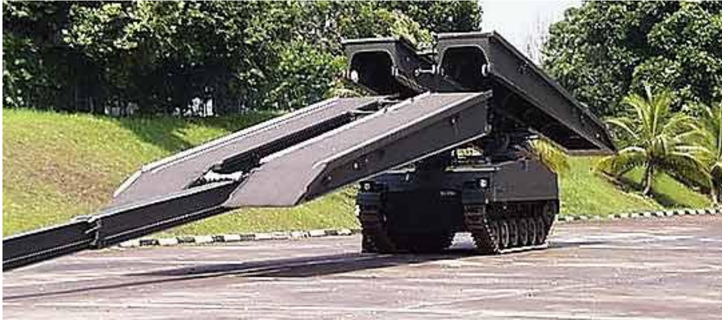
Class 30 Medium Assault Bridge on the Bionix 25 Infantry Fighting Vehicle.
