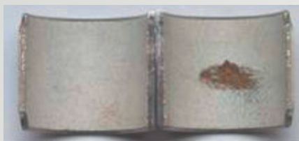
Fig. 35: Local damage caused by cavitation
