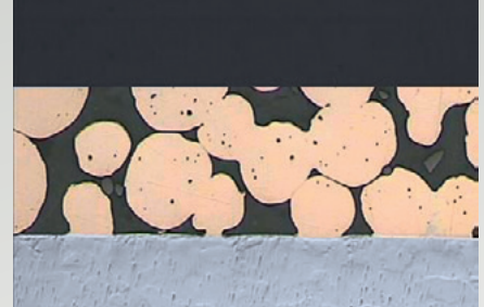
Fig. 9: Condition of sliding surface at end of service life
