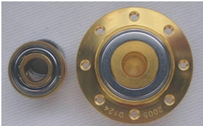
Result of a salt spray test at GRW
