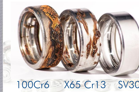
Result of a salt spray test at GRW
