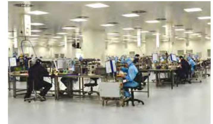
Ball bearing assembly at 1.400m 2 in a clean room class R10.000 ISO-Standard (ISO 14644-1, class 7).
