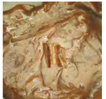
After 1.000 cycles of pressurised steam sterilisation: Discolouration of the surface layer; base oil and thickeners are intact
