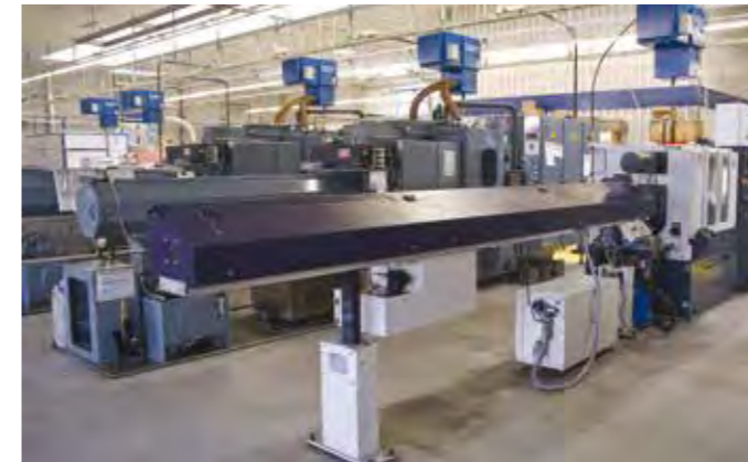
The journey of our products starts in the turning department where our high-precision turning machines produce bearing rings from a variety of steels.
